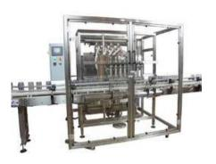
This automatic piston filler by MICRO is ideal for filling liquid, paste in jars bottle, from 30 ml to 1000 ml,. The piston filler provides a highly accurate volumetric fill in that the same amount of product enters and exits the piston cylinder each fill cycle. Automatic piston filling machines will use a power conveyor and one of several indexing systems - from pin to starwheel or screw indexing - to align bottles under the fill heads.
