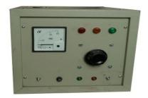
The equipment (Transformer Oil Testing Kit) consist of two High Voltage Coils having Starting winding at earth potential. The High Voltage Transformer is designed for testing Duty only. The equipment is made for testing transformer oil as per IS Specification. Regarding Transformer Oil and Electrode shape.
