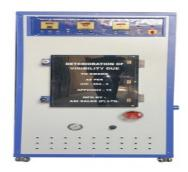
Smoke Density Apparatus offered meets demands of measuring optical density of smoke upon certain thick specimen. Some of its features include:
